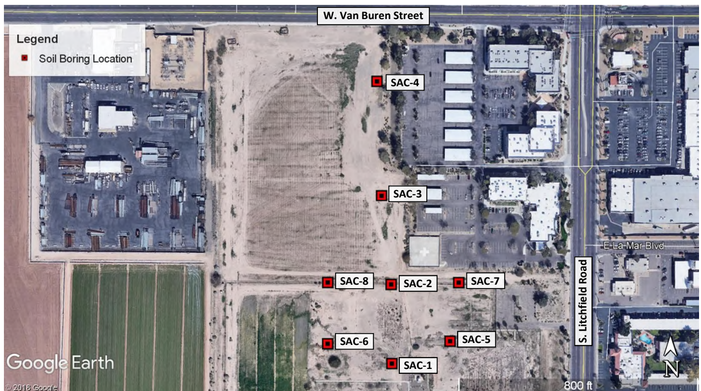
EPA-Approved Soil Boring Locations
